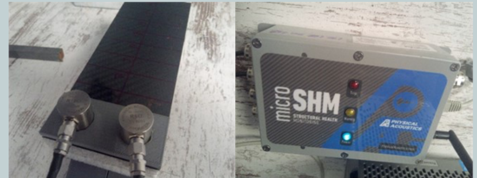
Fig. 1 – Overview of the experimental layout with specimen and sensors; mistras micro-SHM wireless AE acquisition system
