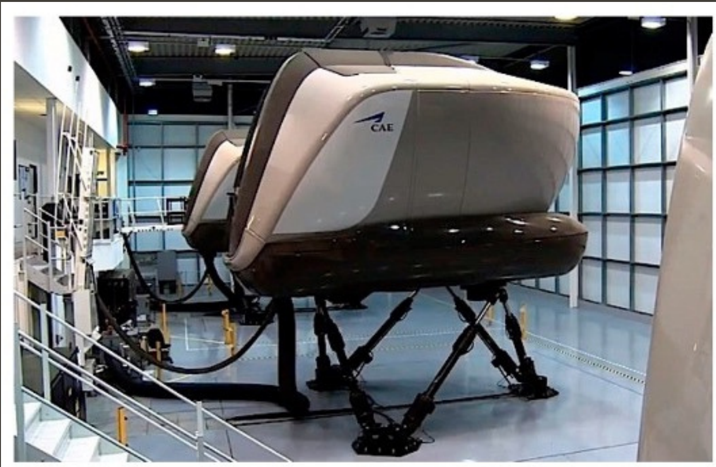
Fig. 3 Integrated CAE 7000XR flight simulator
